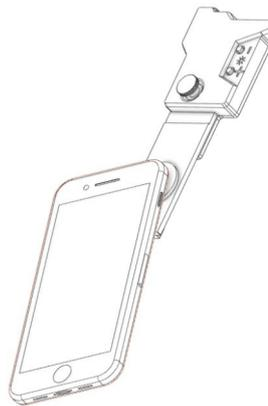
Place the lens tile on the subject to observe. Keep DIPLÉ Lux in one hand, like a magnifying lens, and the phone on the other hand. With the camera-app on, move the phone toward the centre of the black rubber ring and get in contact with it. Slightly tilt the DIPLÉ Lux, or use the elevation screw in the tile to find the right working distance. Change the light intensity with the buttons + and -.
